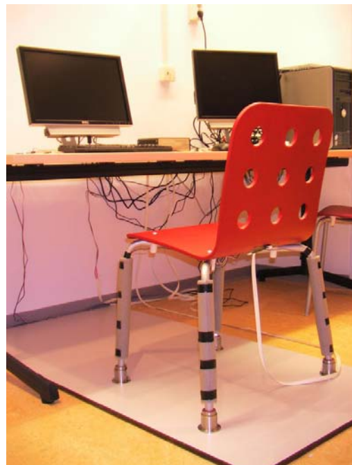
Figure 1: Pressure sensitive chair used for the measurement of people's changes in sitting position.
