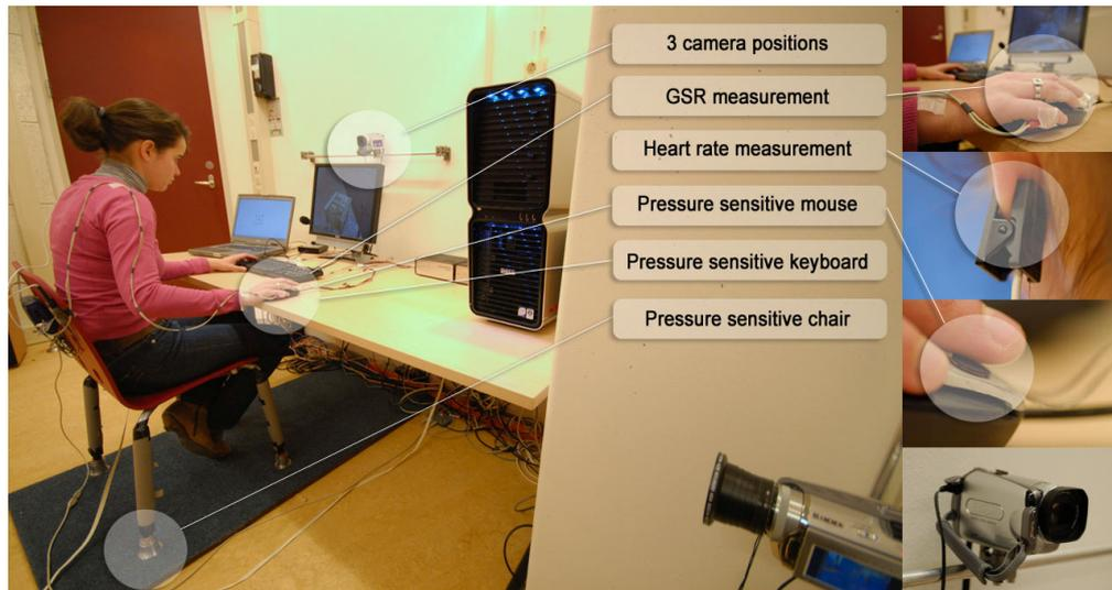
Figure 1: Measurement systems as used in the experiment.
